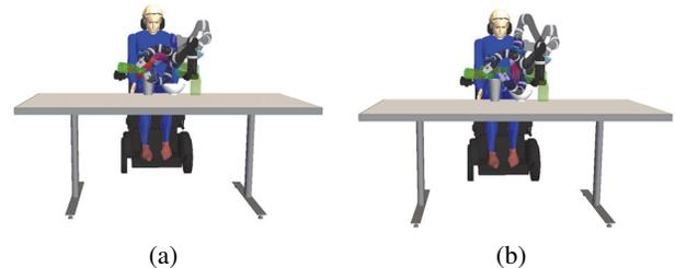
Figure 5: A disabled user moving a bottle using a robotic arm in the presence of obstacles. The trajectory of the arm moves between “safe” and “risk” regions where the bottle is visible (colored green) and non-visible (colored red) to the user, respectively. Snapshots are taken at intermediate points along the path. (a) Shortest path. (b) Minimal-cost path.
